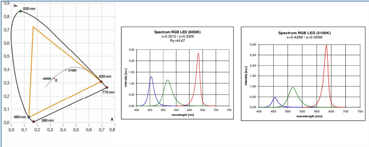
Figure 10: a) achievable chromaticity coordinates within CIE 1931 diagram for RRGB LED
