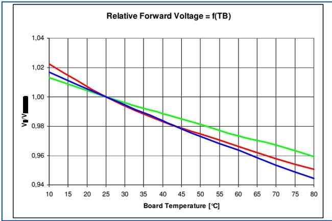
Figure 2: Relative forward voltage versus LED board temperature  $T_B$  for red, green and blue chips (ACULED)
