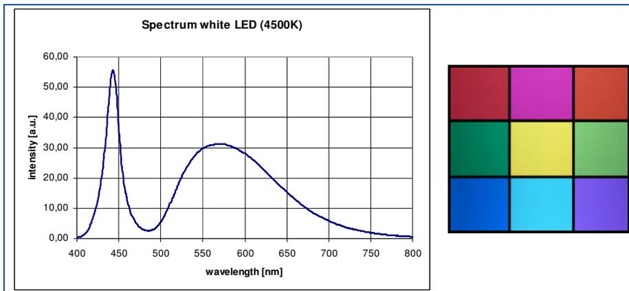
Figure 8: a) spectrum of a cold white LED
