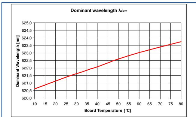
Figure 4: Change of peak wavelength vs. substrate temperature  $T_B$  for the chips of an RGYB-LED
