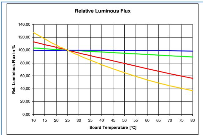
Figure 3: Change of relative luminous flux vs. board temperature  $T_B$  for the chips of an RGYB-LED
