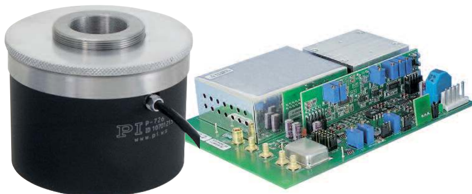
High dynamics PIFOC® objective scanner and OEM controller. The power supply of the controller is usually integrated directly on the circuit board, the same applies to open OEM versions. The operation of the piezo system then only requires a stabilized voltage of 12 or 24 V.
